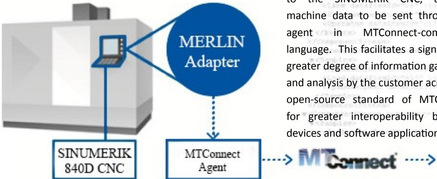
This schematic illustrates the typical scenario for a machine tool control modification at an end-user, where the Memex Automation software is added to the SINUMERIK CNC, allowing machine data to be sent through an agent in MTConnect-compatible language. This facilitates a significantly greater degree of information gathering and analysis by the customer across the open-source standard of MTConnect for greater interoperability between devices and software applications.
